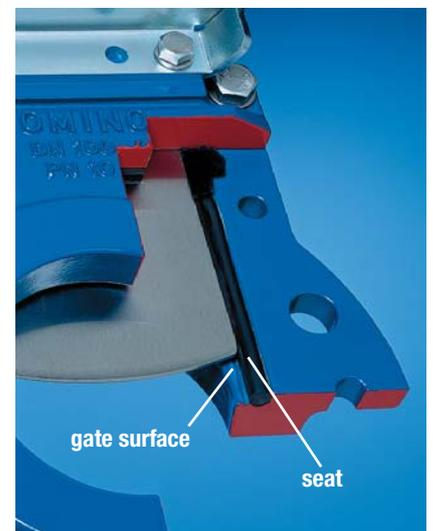
**Bidirectional shutoff** is achieved by the lateral gate surfaces and the elastic seat which is integrated in the body.
